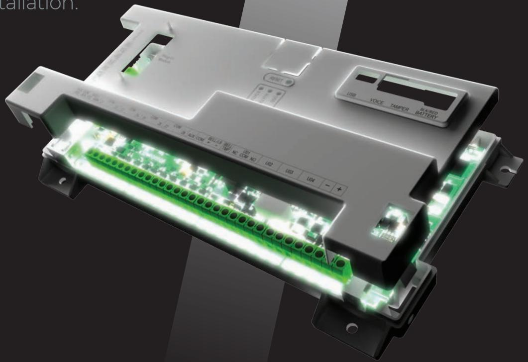
The new LightSYS+ is RISCO's flagship hybrid alarm panel, combining the features and benefits of both LightSYS 2 and ProSYS Plus into one high-powered security system. It is designed to protect any size or type of Grade 2 or Grade 3 installation - enabling up to 512 zones in one single panel!
